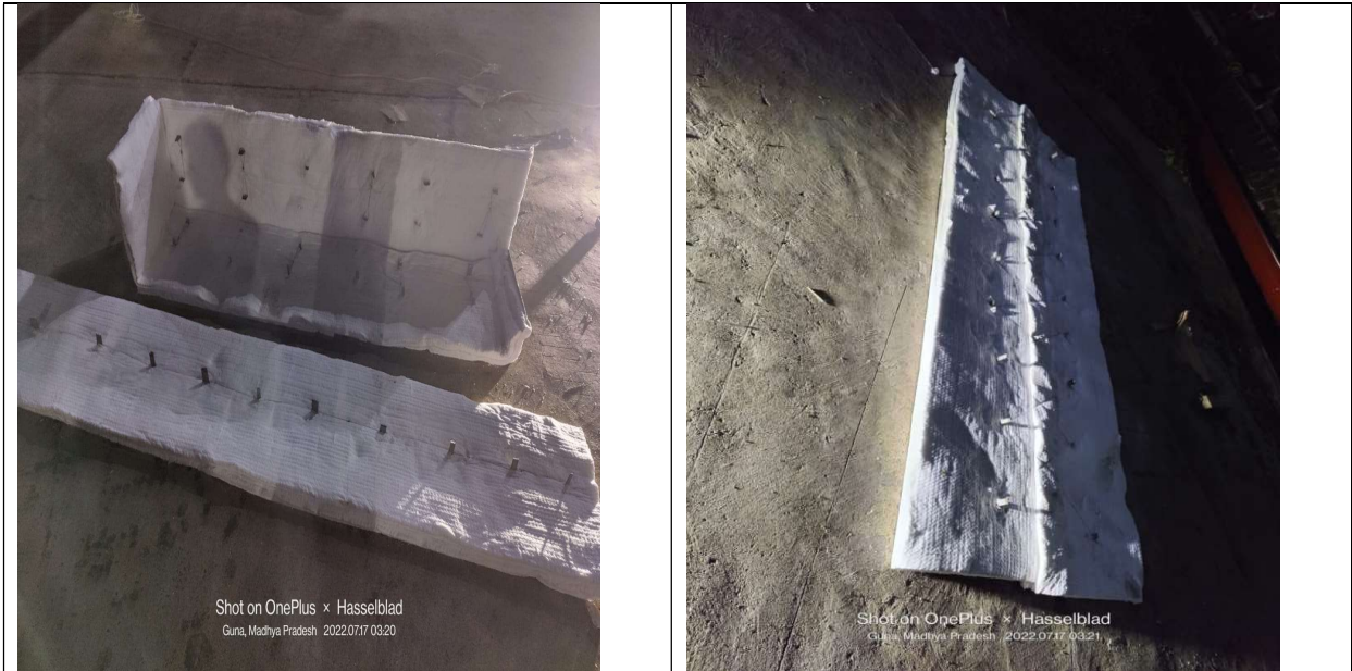
Inconel plate & Box with Cerawool insulation
